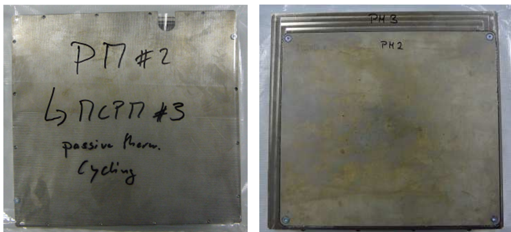
Figure 8 : Top and bottom views of one the fonctionnal MCPM manufactured in WP2.1 and delivered to technological validation test campaign (WP4)
