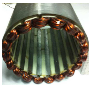
Figure 37 : CREAM motor rotor and stator parts
