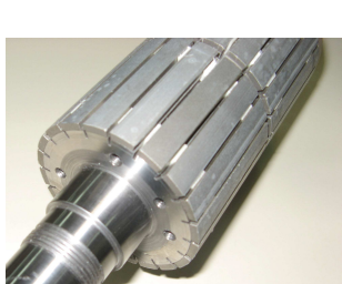
Figure 37 : CREAM motor rotor and stator parts
